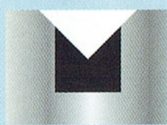
面取り部への座ぐり加工 Spot facing after chamfering part
